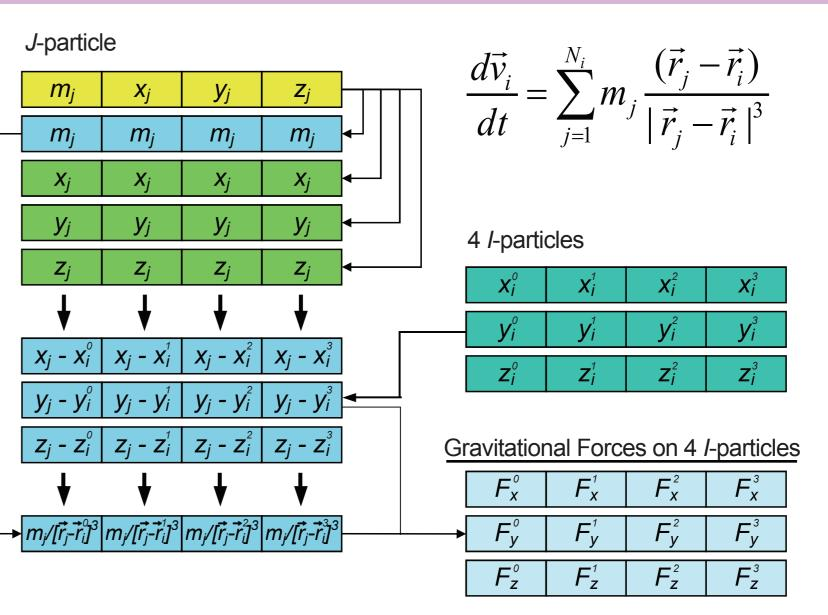
18.3GFLOPS / core is achieved on Core 2 Duo (2.4GHz) processor
