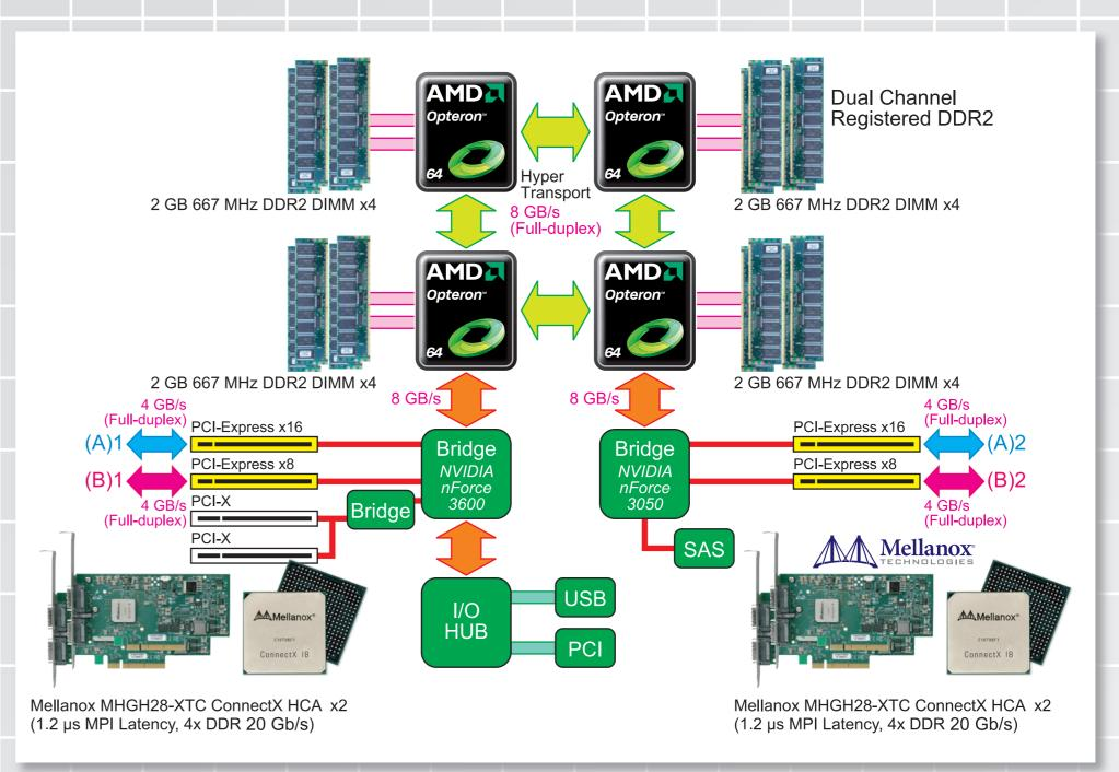
Each computation node is equipped with a 4-socket quad-core Opteron (AMD Barcelona, 2.3 GHz) in a 16-core shared memory configuration with a peak performance of 147.2 GFLOPS. To support such a high-performance node, a quad-rail 4xDDR Infiniband HCA is employed with 16 GB/s (bidirection) of communication performance.
