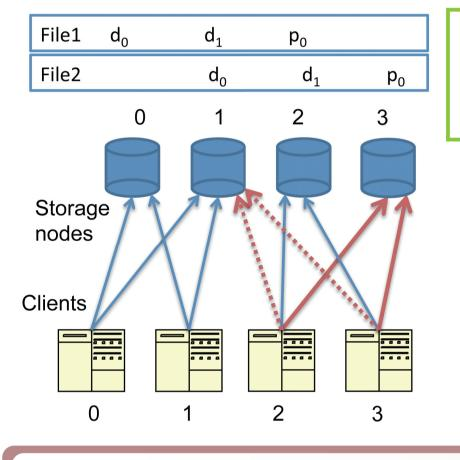
Network of storage node #1 is congested when all clients access the files concurrently. This congestion is avoided by the proposed method, which uses the redundant data to disperse the traffic.
